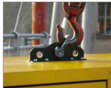
▲ Central lifting eye Crochet de levage central
